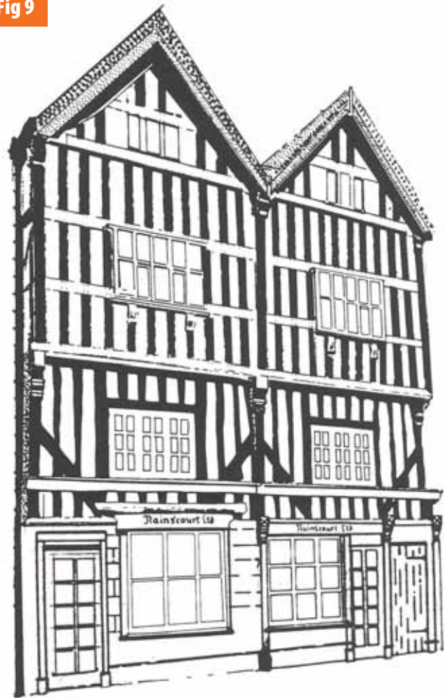
Early nineteenth century shopfront in sixteenth century building with traditional hand painted timber fascias and sub-divided traditional glazing providing for a lively display
