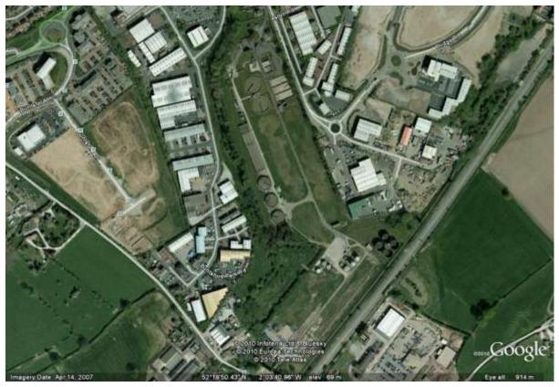
7.3.19 This is the largest STW in Bromsgrove District. It treats flows from the Bromsgrove Town Drainage Area. Treatment is provided by a diffused air activated sludge plant. Summary information for the works is shown on Table 7-7.
