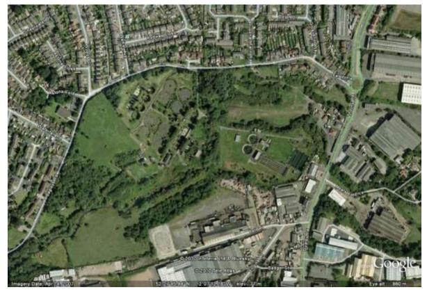
7.3.26 This large STW treats flows from a substantial area around Stourbridge to the west of Birmingham including a small area in the northwest (Hagley) of the Bromsgrove District. Treatment is provided by a diffused air activated sludge plant. Summary information for the works is shown on Table 7-9.
