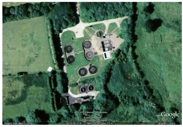
7.3.10 Astwood Bank STW treats wastewater from a small part of the Redditch Rural Drainage Area by means of re-circulating filters. It is situated on the south east boundary of Redditch Borough. Summary information for the works is shown on Table 7-4.
