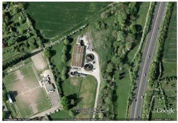
7.3.13 This STW treats flows from the Alvechurch sub-area of the Bromsgrove Rural Drainage Area in the east of the District. Treatment is provided in an oxidation ditch. Summary information for the works is shown on Table 7-5.
