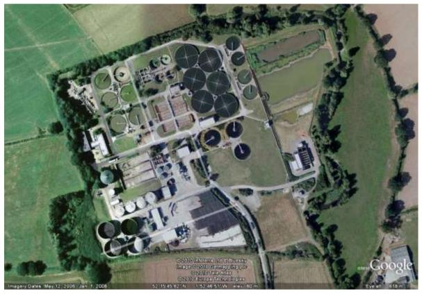
7.3.1 This is the largest STW serving Redditch Borough and uses the activated sludge process with diffused air aeration. It treats flows from the Spernal Drainage Area that serves the majority of the towns of Redditch and Studley. The Works lies outside and to the south east of Redditch Borough. Summary information for the works is shown on Table 7-2.
