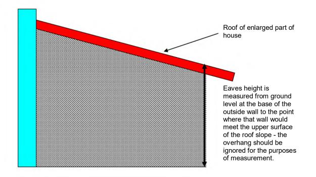
The following example shows the side view of an extension with a pitched roof:
