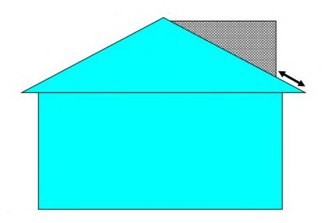
Minimum of 0.2m from eaves to edge of the enlargement to be measured along the roof slope from the edge of the enlargement to the outer edge of the eaves. The enlargement cannot overhang the outer face of the wall of the original house.
