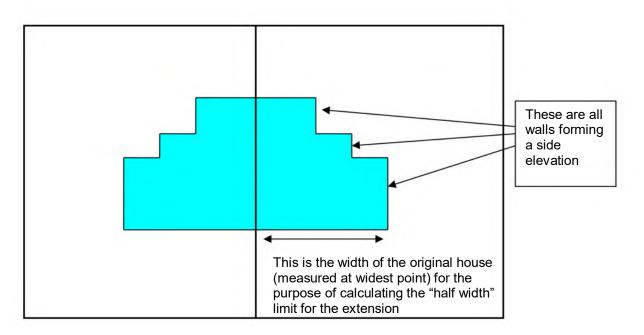
Where an extension is beyond any side wall, the restrictions in (j) will apply. Any extension can only be a single storey, must be less than 4 metres in height and can
