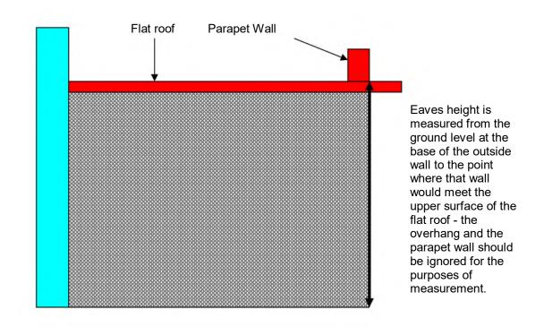
Where the existing house has eaves of different heights, then the restriction on the height of the eaves for the part of the house enlarged, improved or altered is measured against the highest level of eaves on the existing house. However, where a house is built on sloping ground, the height of the eaves on the existing house should be measured in terms of the elevation from which any extension of a house is to be made.
