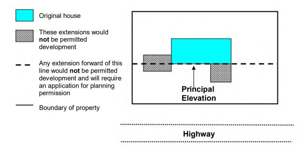
The principal elevation could include more than one wall facing in the same direction - for example, where there are large bay windows on the front elevation, or where there is an 'L' shaped frontage. In such cases, all such walls will form the principal elevation and the line for determining what constitutes 'extends beyond a wall' will follow these walls.
