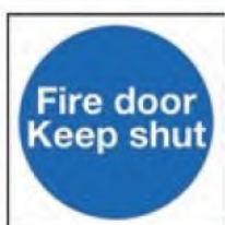
Figure C9: Notice for fire resisting doors
